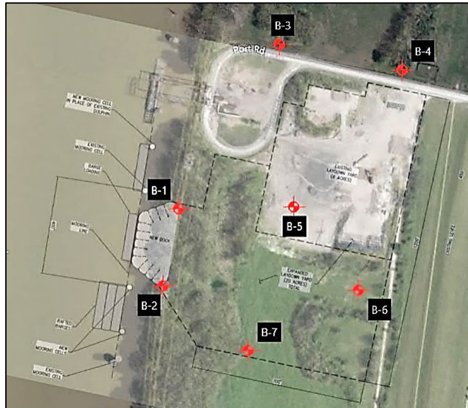
Figure 2-1: Geotechnical Boring Locations shown in red
